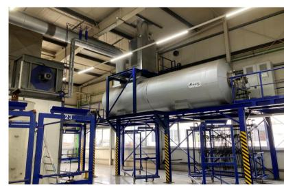
The compact thermal recuperative oxidisers are the preferred units for the cleaning of industrial exhaust air with high concentrations of VOC's which occur mainly in printing, coating, laminating and impregnating processes.
