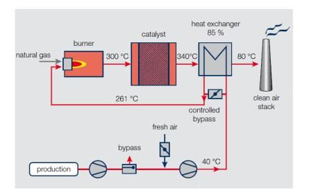
Up to 85 % of the heat energy can be used for preheating the exhaust air by the use of high efficiency, plate-type heat exchangers. The subsequent low clean air temperature enables catalytic incinerators to function economically without any secondary waste heat recovery system.
