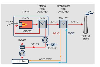
heat exchanger, in which each individual pipe is fitted with its own expansion joint, enabling a waste heat recovery efficiency of up to 76 %.
