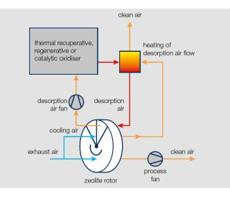
Depending on the type of VOC, the composition and operation mode a concentration ratio of up to 1:50 is possible. In a second process step, the desorbed air is treated in a thermal, regenerative or catalytic oxidation system.
