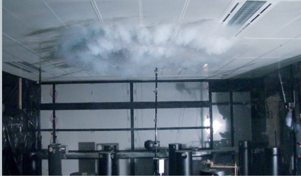
Principle sketch of the mode of operation, air flow pattern made visible by smoke
