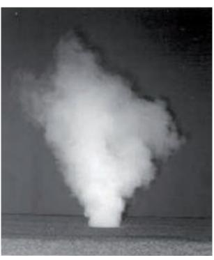
Figure 5: Jet pattern of floor twist outlet made visible with smoke tracer
