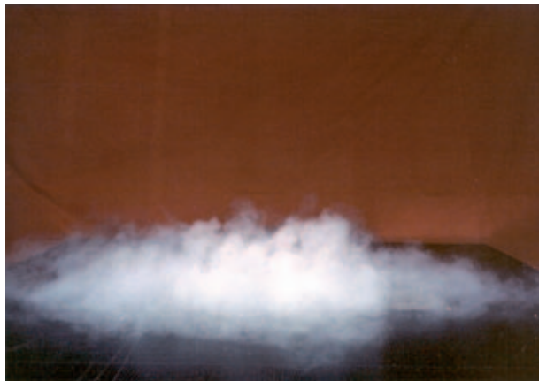
Figure 4: Low-turbulence horizontal, radial jet dispersion, made visible with smoke tracer
