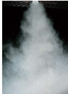
Air jet pattern of RA-V below: horizontal discharge (cooling mode) left: vertical discharge (heating mode)
