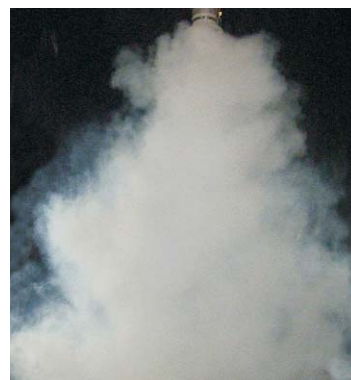
Air jet pattern of RA-V2 top: cooling mode bottom: heating mode
