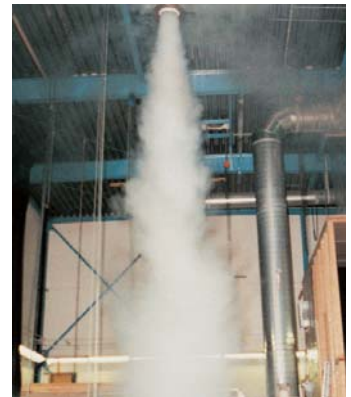
Air jet pattern of DD-VG (heating mode)
