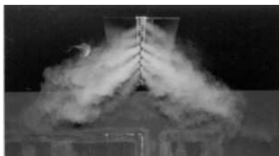
Fig. 4: Air jet pattern made visible with smoke tracer
