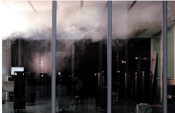
Figure 8: Cooling mode, supply air temperature 16 to 21 °C
