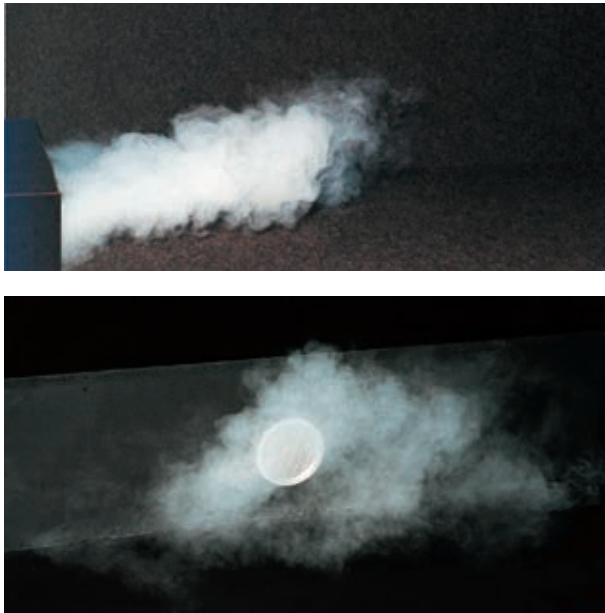
Fig. 7: Jet pattern made visible with smoke tracer top: Linear step displacement outlet bottom: Circular step displacement outlet
