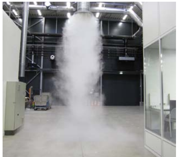
Fig. 6: Vertical discharge from a great height, jet pattern made visible by smoke tracer
