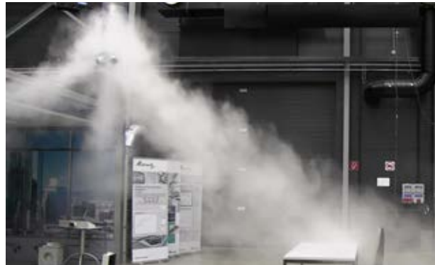
Figure 5: Displacement mixing flow with focused nozzle position
