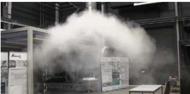
Figure 1: Flow pattern visualised by smoke; displacement mixing flow
