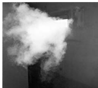
Jet pattern made visible with smoke tracer
