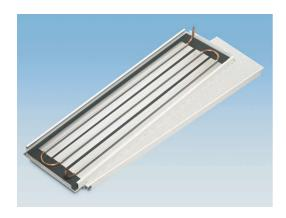
The contact cooling ceiling system KKS-3/LD is designed for combination with plane metal acoustic ceilings from various manufacturers to produce radiant cooling or heating ceilings or walls. The permanent large-surface contact between the cooling element and the ceiling tile is done with adhesive.
