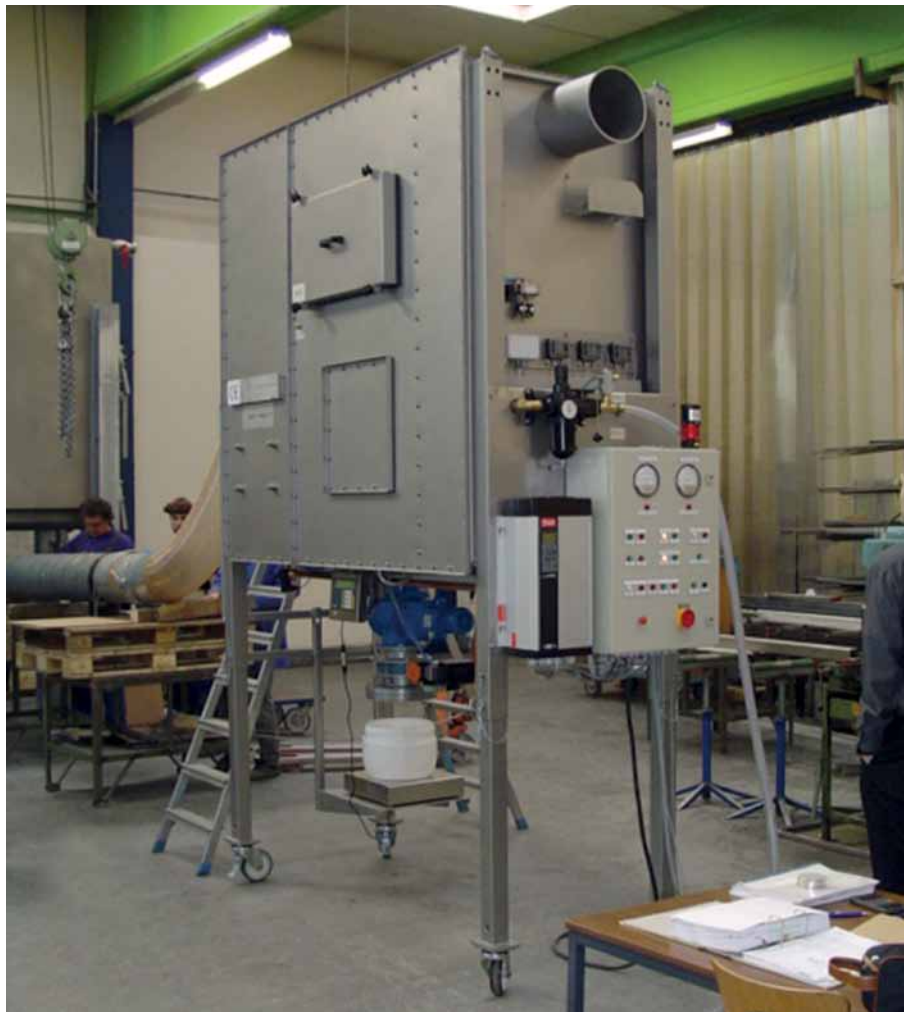
FAT Factory acceptance test M-RHF | hightec 2x1 RH13-1x1 H13
