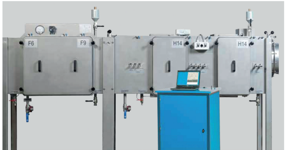
HEPA filter system, type SCF hightec Triple S with pre-filters and two stages of HEPA filters H14
