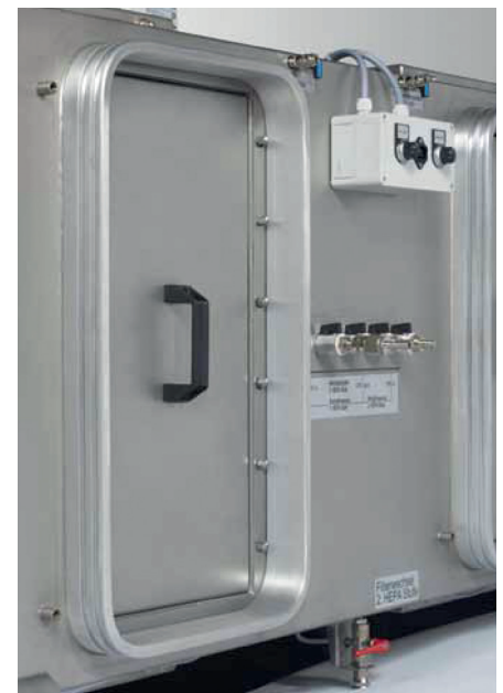
Special collars with sealing grooves acc. to DIN 25 466 supp. 1 ensure gastight seat of the plastic bag for safe bag-in bag-out changing of filter elements
