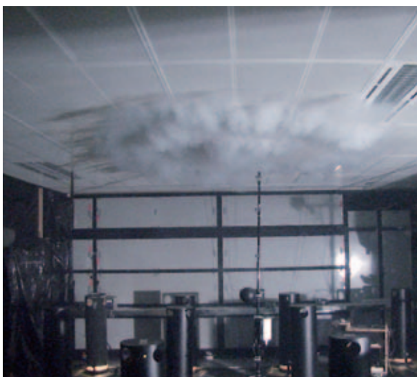
Air flow pattern of the PDK and PCK
