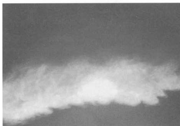
Fig. 7: Low-turbulence horizontal jet spread made visible by smoke tracer; the photographs show the air flow at various points in time after discharge
