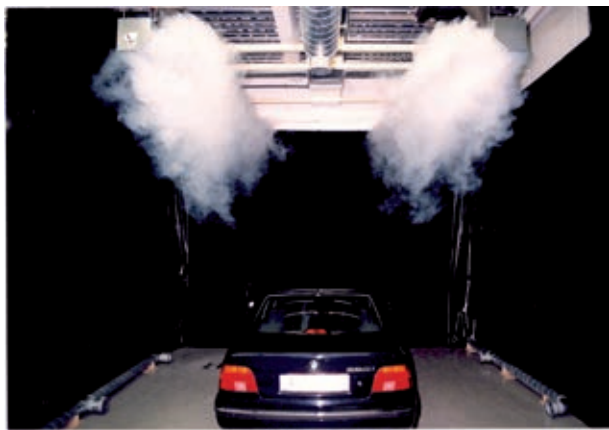
Figure 7: Semi-trapezoidal displacement outlet in a test room of the automotive industry
