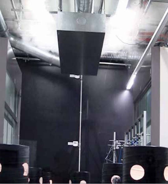
Visualization of air flow using artificial smoke
