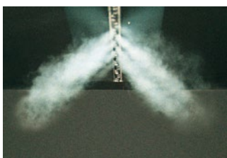
Air jet pattern, discharge angle approx. 45°
