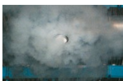
Air jet pattern, horizontal discharge (cooling mode)
