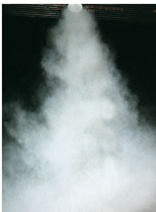
Air jet pattern, vertical discharge (heating mode)
