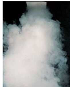
Air jet pattern of Q-DN and Q-DV left: cooling mode; right: heating mode (only Q-DV)
