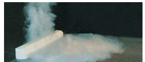
Air jet pattern of Q-SH (when heating)
