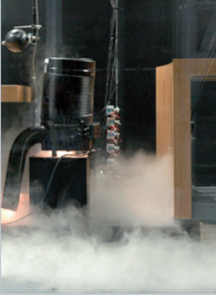
Lab testing of displacement ventilation in a parliament building (State Parliament NRW Düsseldorf)
